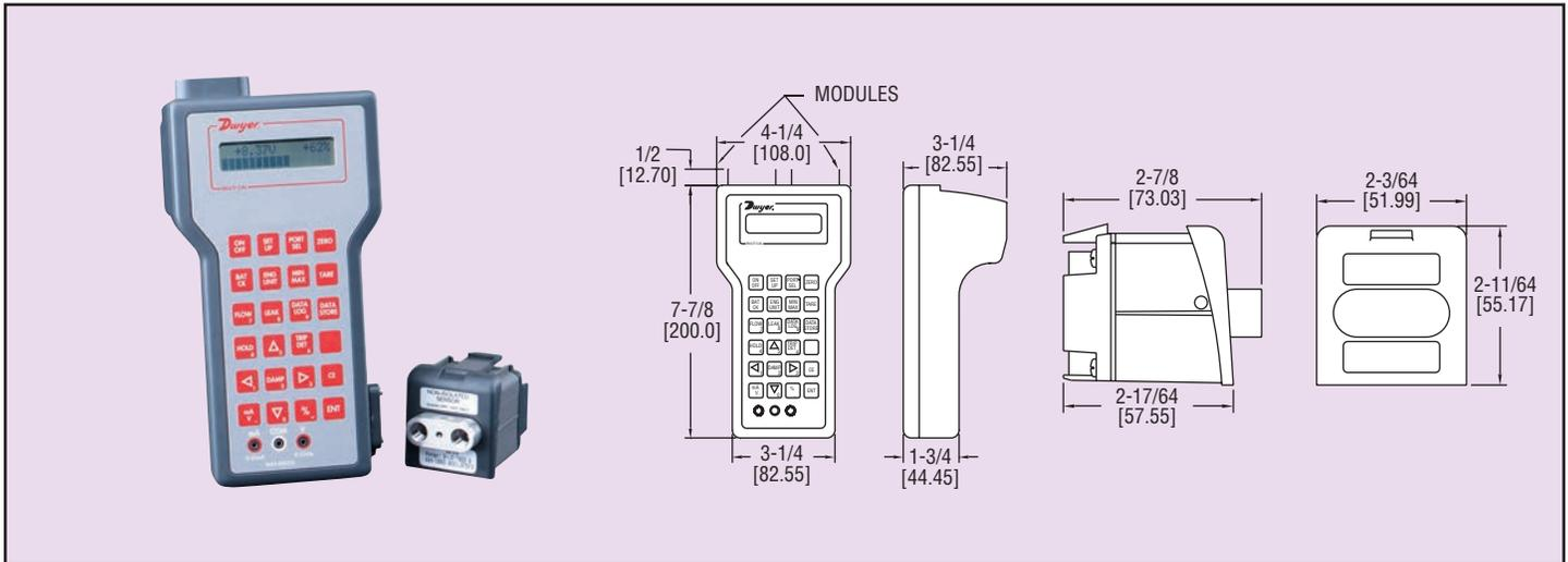
**Series MC Portable Multi-Cal Pressure Calibrator** performs a wide variety of simple and complex pressure based measurement, test, and calibration operations. Modular sensor design allows user to select pressure measurement range for application flexibility. Calibrator can accommodate up to two interchangeable pressure modules (sold separately below) in any combination of range or accuracy.
