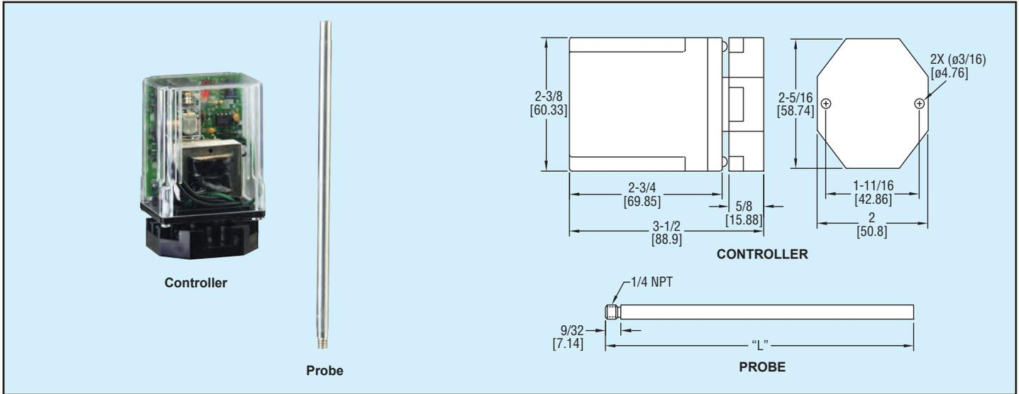
**Control valves, pumps and alarms** with the versatile Series LLC Conductivity Level Controller. Select the required number of probes for single or dual point level detection. Choose probe lengths in 1-foot increments (up to six feet) to adapt the LLC to your specific applications requirements. The LLC features rugged 1/4" (6.3 mm) diameter, SS probes, LED monitoring, surge protection, low voltage sensor and different mounting options.
