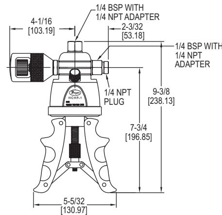
The Series HCHP Hydraulic Calibration Hand Pump utilizes a fully adjustable stroke control that allows for quick priming, easy pumping, and fast pressure generation up to 10,000 psi (700 bar). The ergonomically engineered handles provide extra comfort, while the triple filtration system ensures pump operation in spite of dirty conditions.
